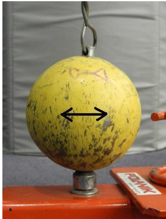
NOT a useful measurement This checks the lateral CG offset, which is not an advantage to the thrower
