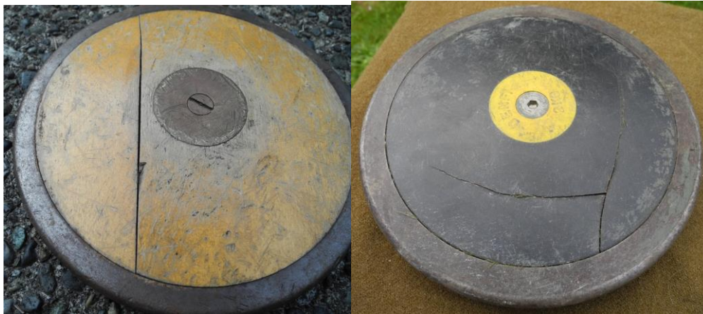
The major cracks in the above discuses will disqualify them.
