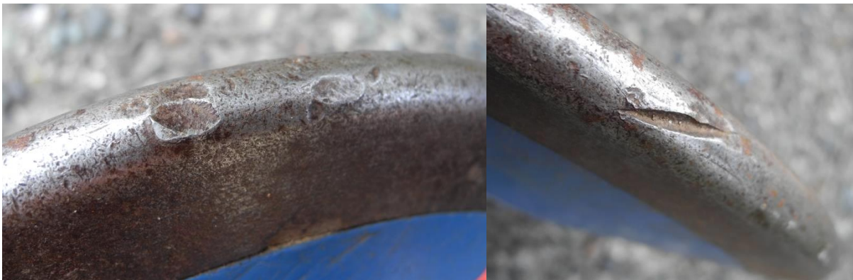
The above gouges and dents can be gripped, and therefore, are not legal. But any rim condition that improves grip is not permitted.
