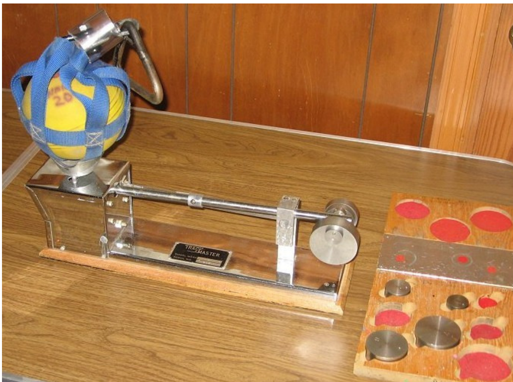
Figure 6: Old Trackmaster Level Scale with Weight
