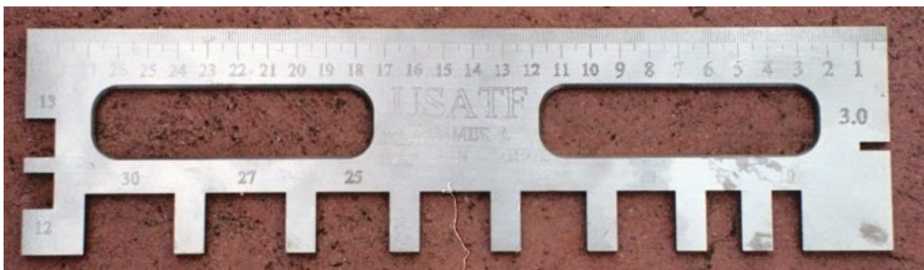
Figure 30: Javelin Contour Gauge used in So. California
