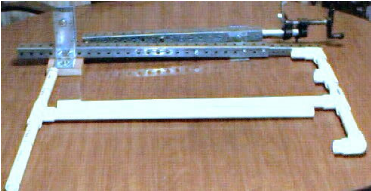
Figure 14: Hammer Stretcher and Length Gauge used in Pacific Association
