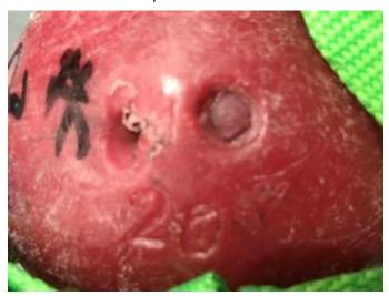
with some pretty big holes (indentations?). If those go deep enough, the lead fill can leak out and cause the shot to become light. If these are thrown onto a turf field, the lead pellets are toxic and need to be removed which is a major problem given the rubber pellets used as infill.
