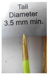
This jav's tail was "sharpened" and then painted over. However, it fits within a 3.5 mm notch. It should be repaired or disqualified
